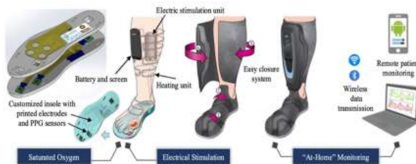
Figure 9. Prototype of the wearable boot device for at-home monitoring of the diabetics' foot ulcers via continuous measurement of the ulcers' saturated oxygen and electrical stimulation treatment [6].
